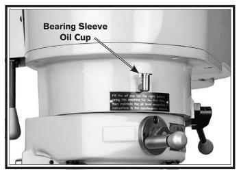
Figure 48. Speed range bearing sleeve.
